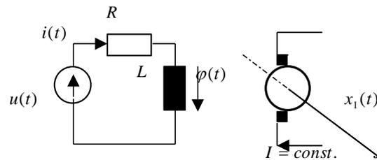
Abbildung 1: A DC electric drive as a model of moving part of the oriented PV system
