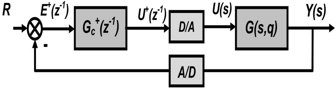
Abbildung 3: A digital closed-loop control system
