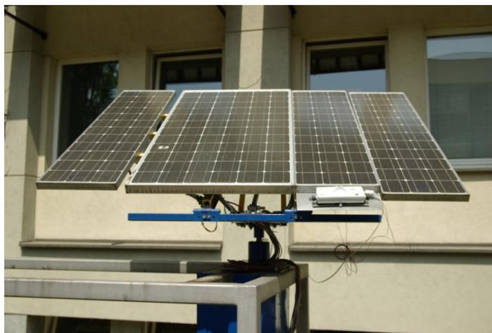
Abbildung 2: An experimental oriented PV system
