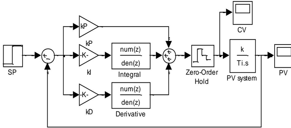
Abbildung 4: The SIMULINK model of the considered closed-loop control system
