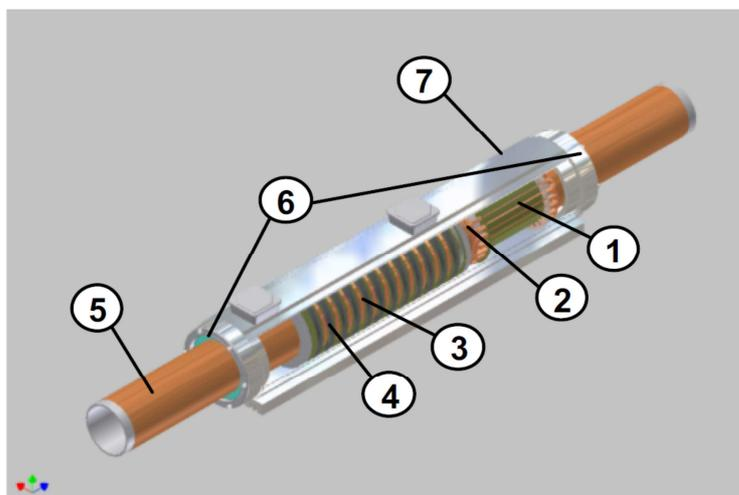
Fig.1. Construction of linear – rotary induction motor: 1 – yoke of stator of rotary module, 2 – winding of rotary module, 3 – yoke of stator of linear module, 4 – winding of linear module, 5 – tubular rotor with conducting copper layer, 6 – bearings system, 7 – casing
