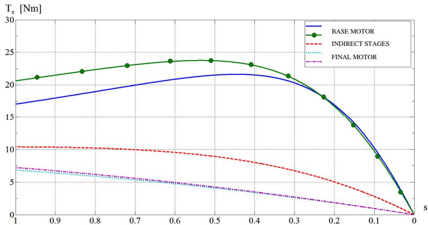
Fig.3. „Transformation of structure” – electromagnetic torque versus slip curve  $T_e = f(s)$  for adequately stages of transformation
