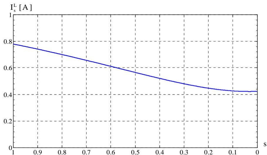
Fig. 7. Stator current versus slip curve  $I_s^L=f(s)$  – module L
