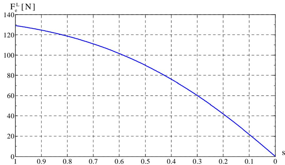
Fig. 6. Electromagnetic force versus slip curve  $F_e^L=f(s)$  – module L
