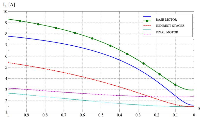
Fig.4. „Transformation of structure” – stator current versus slip curve  $I_s = f(s)$  for adequately stages of transformation
