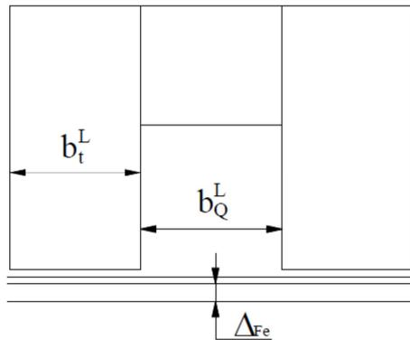
Fig. 5. Dimension of slots and teeth of stator – module L
