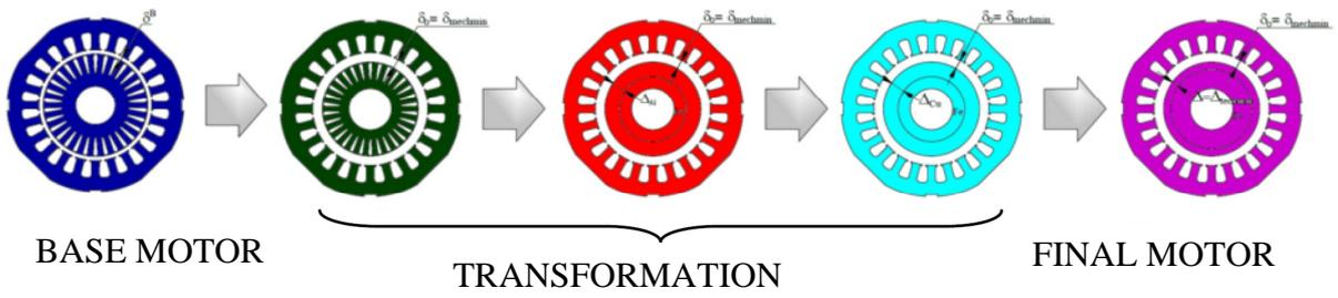
Fig.2. Idea of „Transformation of structure” induction cage motor to rotary module of linear – rotary induction motor
